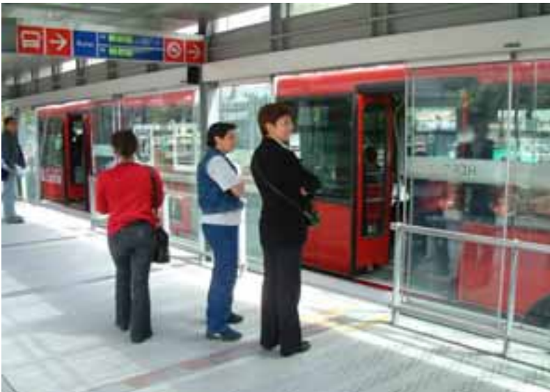
Figure 3.6: Station in Bogota showing level boarding
